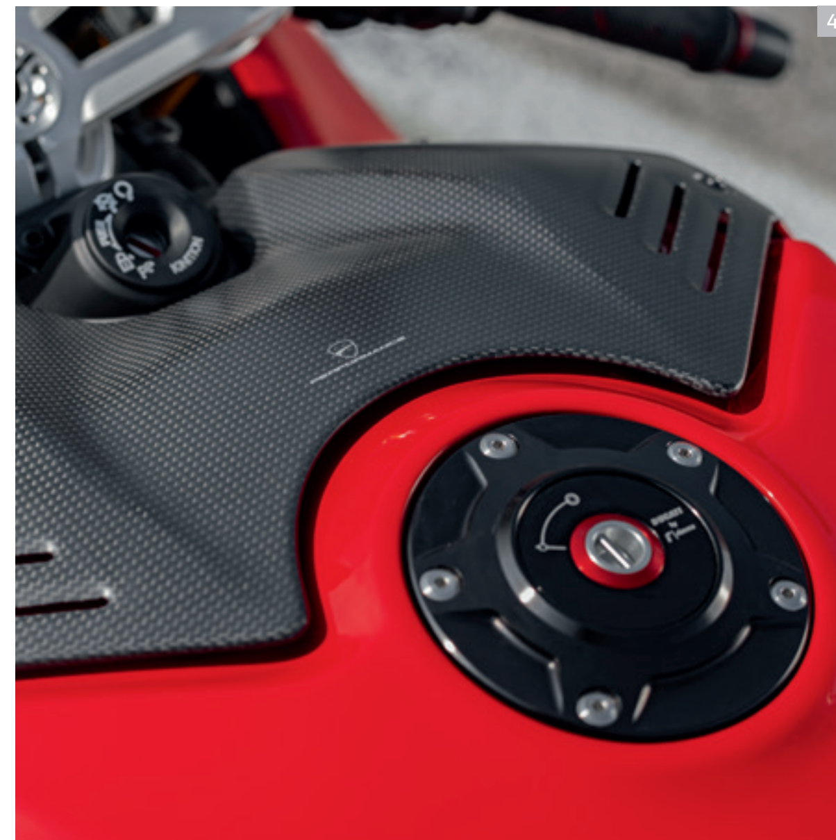
4 Carbon tank cover. Billet aluminium tank cap
