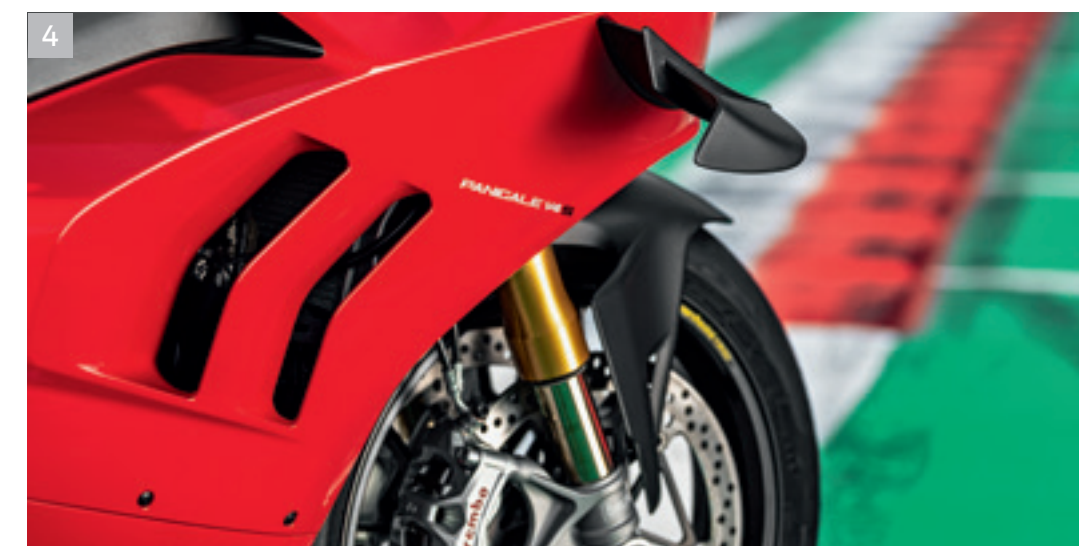
3 Öhlins suspension with Öhlins Smart EC 2.0 control system
