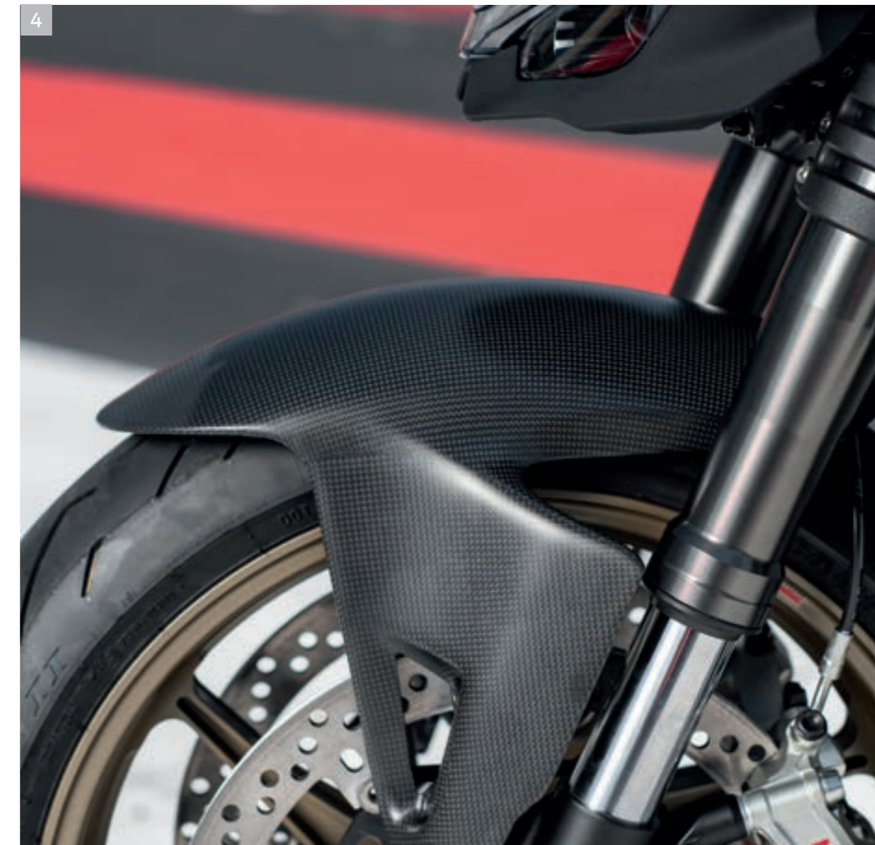
3 Carbon rear mudguard 4 Carbon front mudguard
