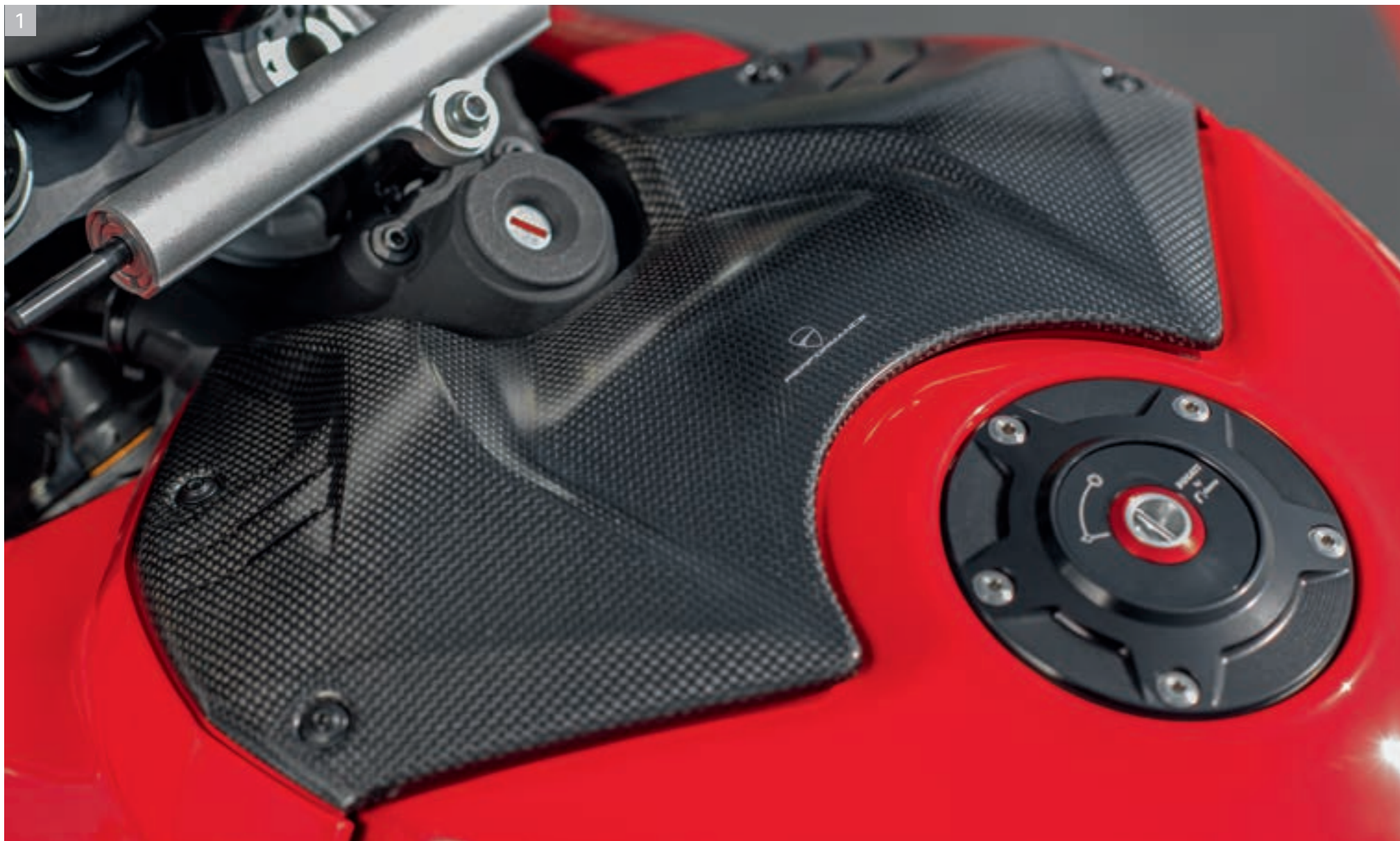
1 Carbon tank cover Billet aluminium tank cap
