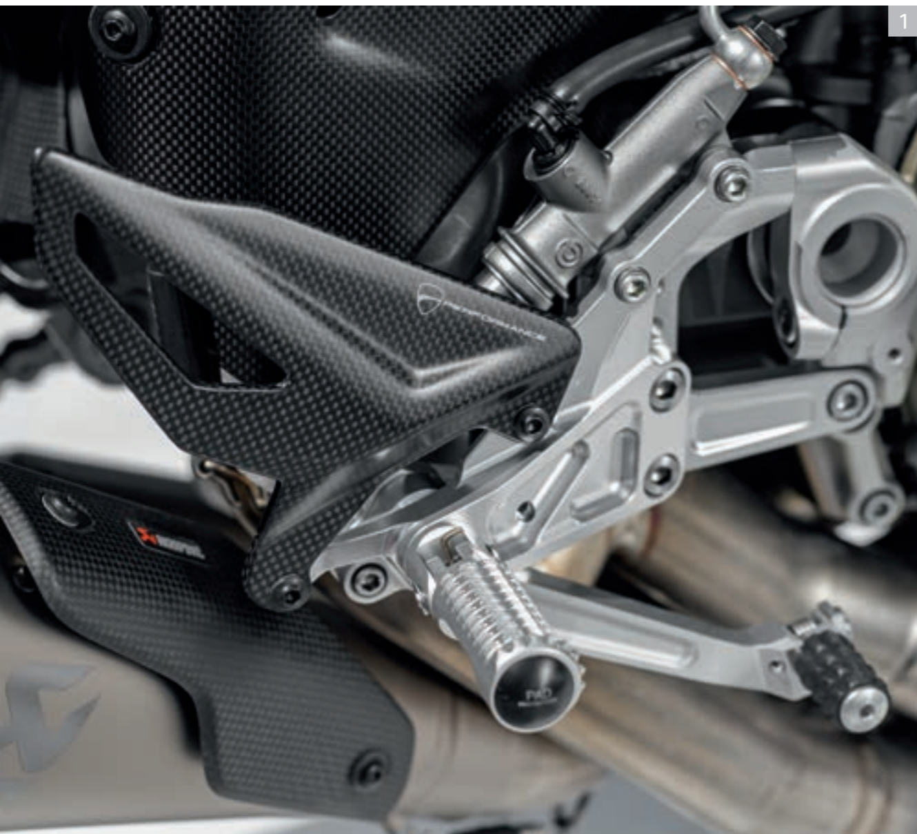
2 Carbon heel guard Adjustable rider footpegs in aluminium
