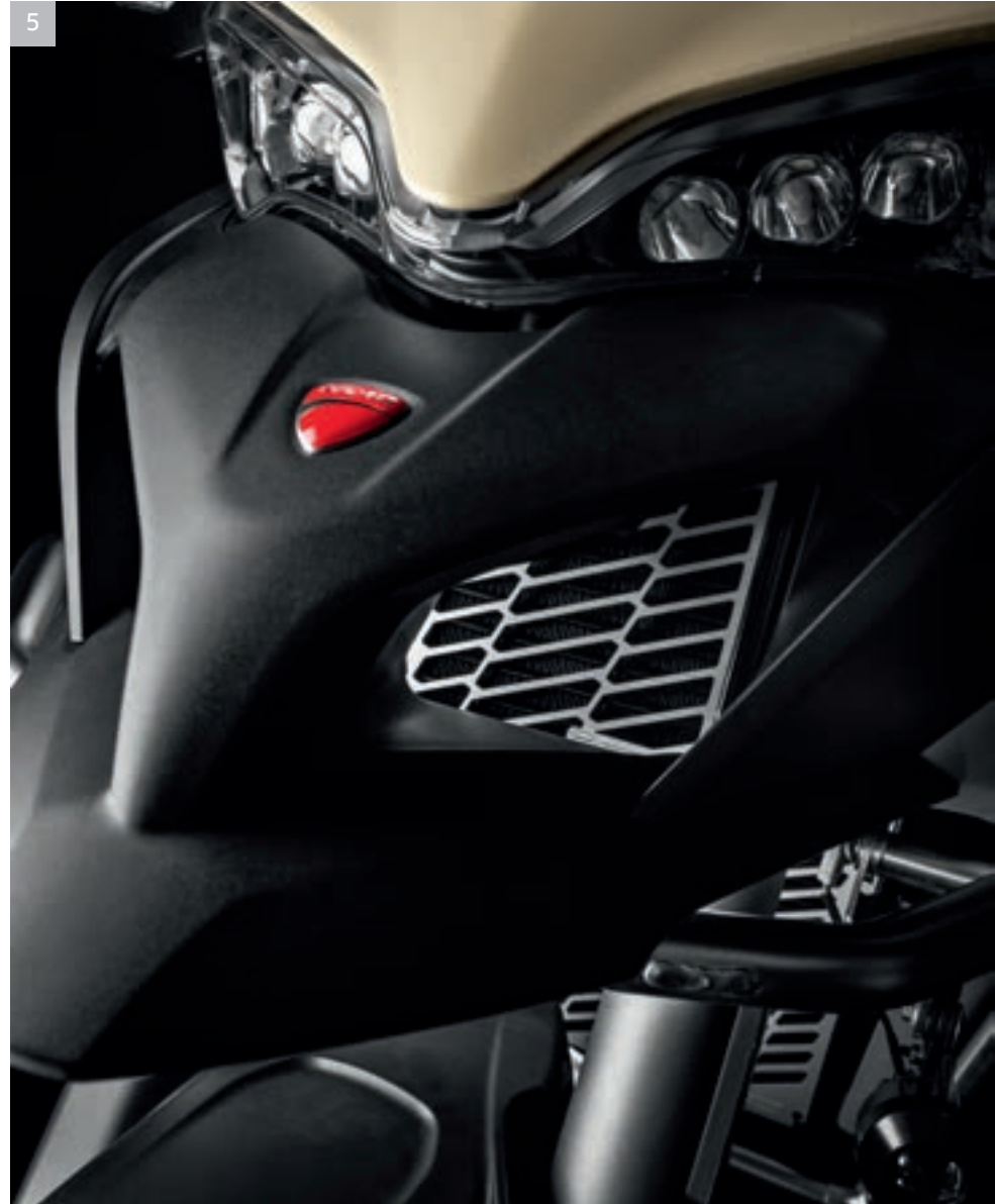
5 Protective mesh for oil cooler
